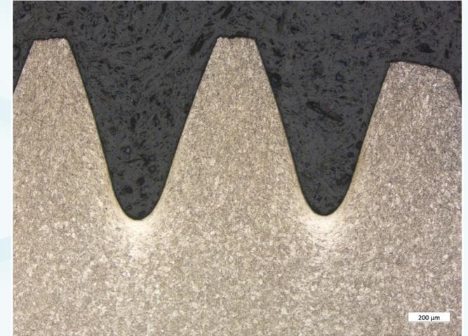
Stainless Steel fastener, external electrolytic etching with 10% aqueous oxalic acid, BF, 50x
